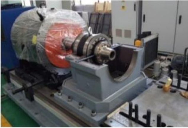
Aircraft shafting bearing testing machine
