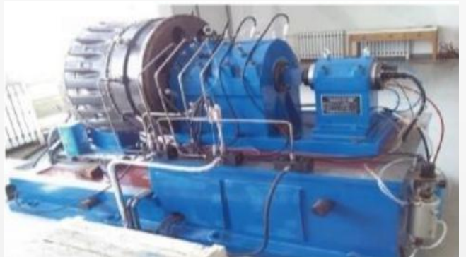
Robot RV reducer bearing testing machine
