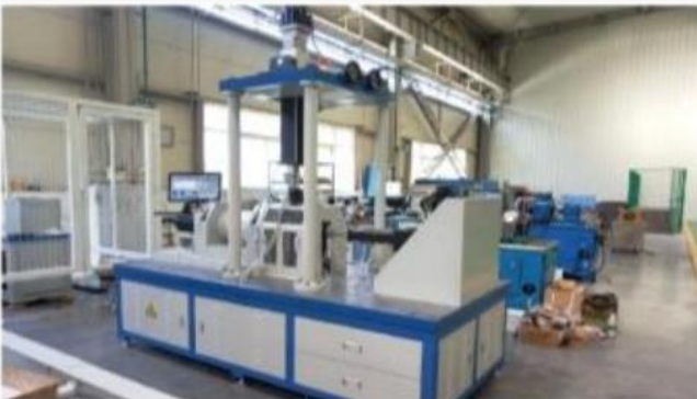
Aeroengine intershaft bearing testing machine
