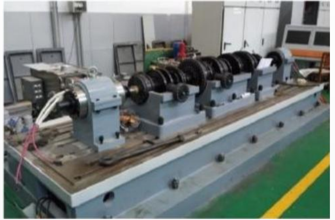
Aviation over clutch dynamic performance testing machine
